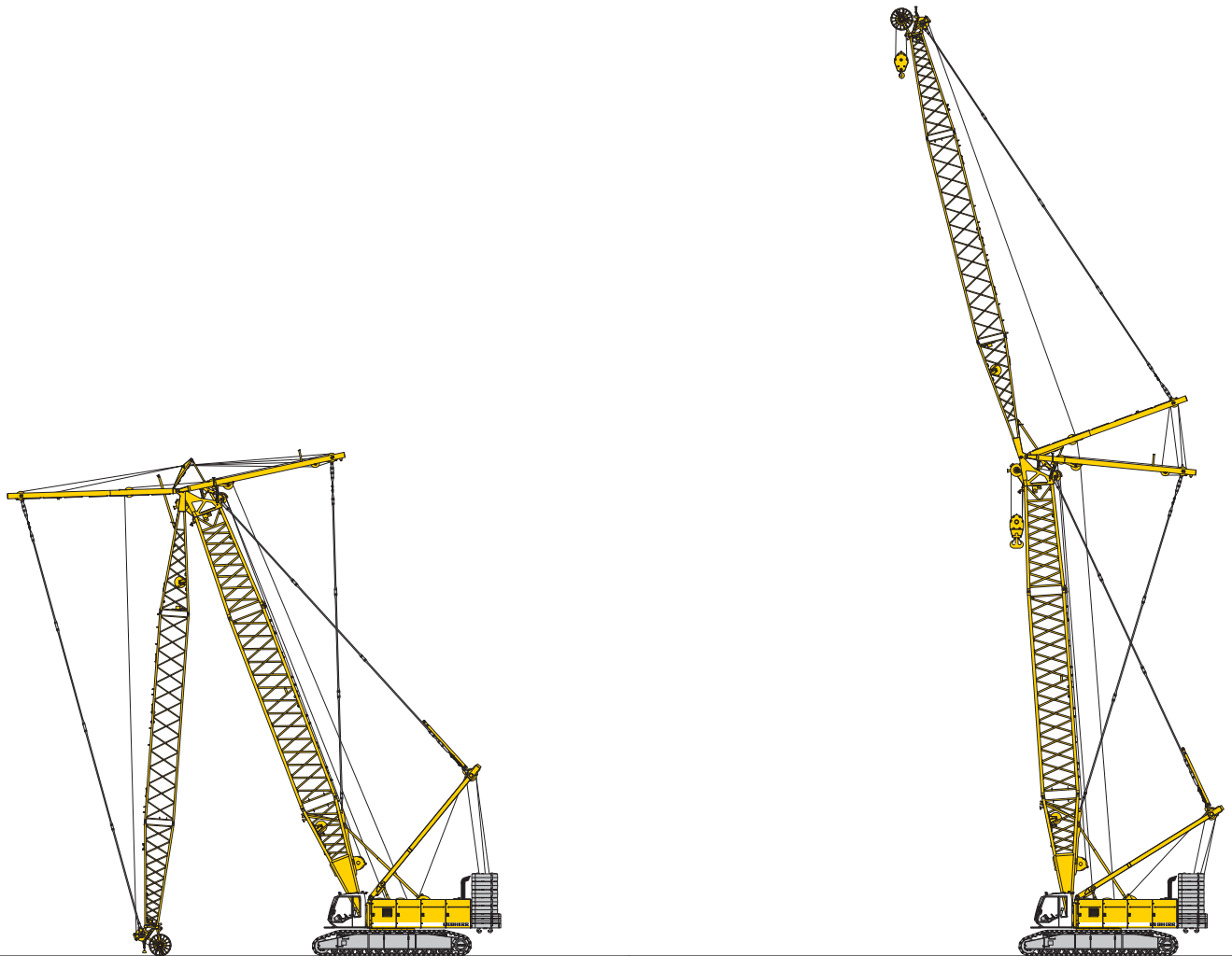
Erecting of main boom and luffing jib
