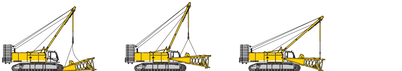
Unloading and assembly of boom foot
